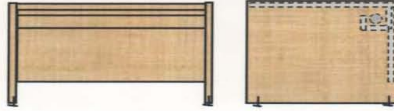
NO.3 L203 COMPUTER TABLE W/ "J" WIRE TROUGH 30" W X 36"L X 28"HIGH.
