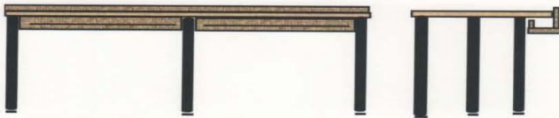
NO.3 L204 COMPUTER TABLE W/ "J" WIRE TROUGH 30"W X 72"L X 28"HIGH. Legs will be 2-1/4" round black metal with adjustable glides.
